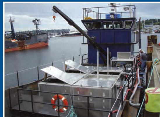
Crab tender *Inaliq* equipped with four portable live holding tanks, titanium chillers and aeration system
